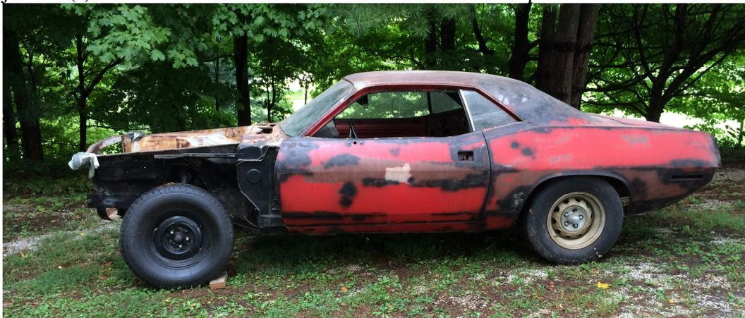
When purchased, the 440-6 Cuda was only a rolling body with an automatic transmission hanging in it without engine. The entire front doghouse was gone and had been sanded down so surface rust and primer over some original faded red paint remained. Though not much to look at, it was structurally sound. What attracted me was that the main body was surprisingly solid with minimal rust problems except for the trunk floor. And it was a 440-6BBL Shaker car!
