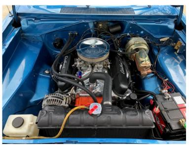
Wedan Performance had a 318 with 4 barrel intake and carb that was taken out of a Mopar (the owner had a 340 installed) and another 904 transmission. So we decided to have the 318 and other 904 done the way we wanted. The 318 had an Edelbrock intake manifold and Edelbrock Performer 4 barrel 600 CFM carburetor.
