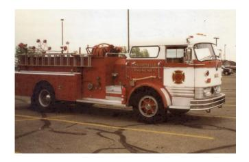
Another Hobby in 2000 – our 1965 Mack Fire Engine 11 litre Turbo Diesel with 1250 GPM Pump
