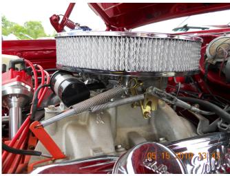
I have replaced the cooling system (Griffin aluminum radiator), ignition system from single points to a Mopar Performance system, fuel system utilizing a new Edelbrock 750cfm carburetor, high volume fuel pump, and fuel lines from Earl's – Indy.
