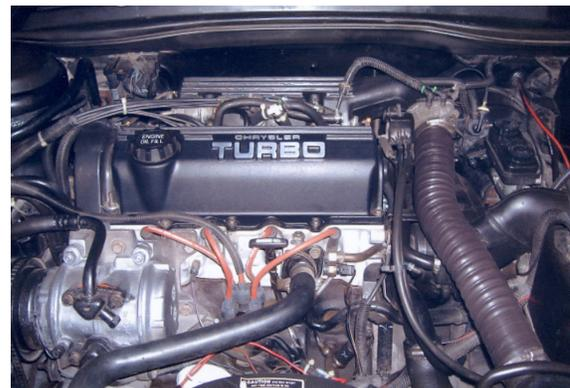
The VNT (variable nozzle turbo) Turbo is what makes these cars so rare. Carrol Shelby came up with the system in 1989 on his CSX VNT Shadows. For 1990 Chrysler decided to use the set-up on their production
